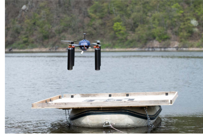
Fig. 1. UAV landing on USV in real-world experiments.
