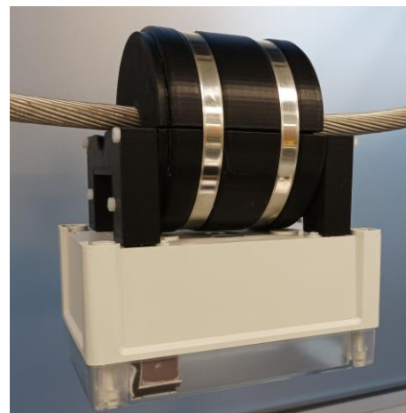
Fig. 4 Gateway prototype with magnetic energy harvester on a test power line at the Circe Electronics Laboratory.
