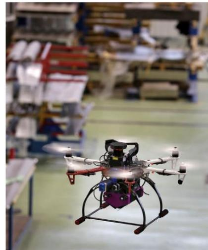
**Figure 1:** Aerial robot performing autonomous light object delivery in the Centro Bahía de Cádiz (CBC) Airbus D&S factory.
