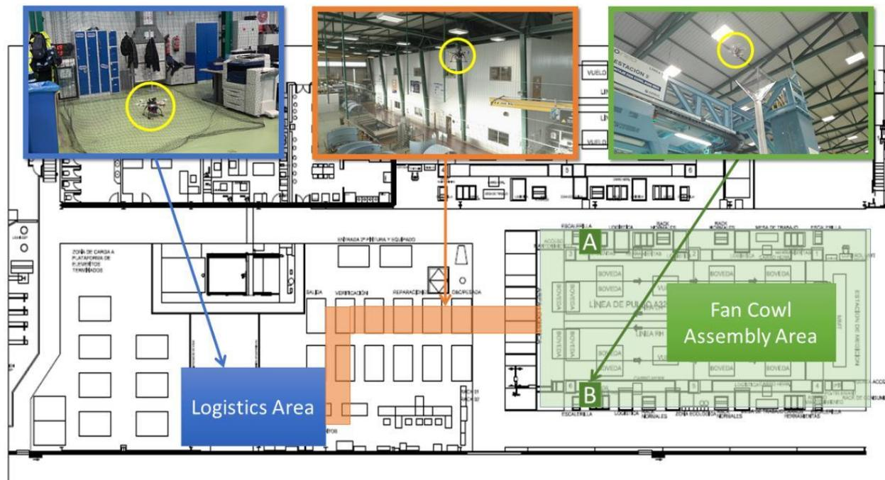
**Figure 10:** Layout of the CBC Airbus D&S factory showing the storage center at the logistics area with the take-off/landing location (in blue), the flying corridor (in orange) towards the fan cowl assembly working area (in light green), which includes hoppers A and B for light object delivery (in dark green).
