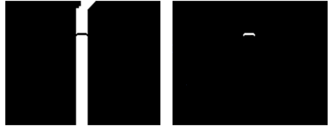
Fig. 8: Frame after the application of the Arc mask (left). Extracted pixels belonging to the path (right).
