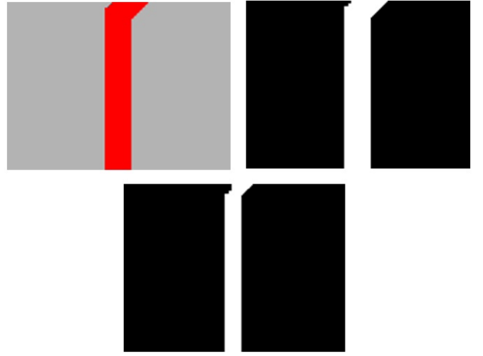
Fig. 6: Original frame (upper left), converted and binarized frame (upper right), and eroded frame (lower).
